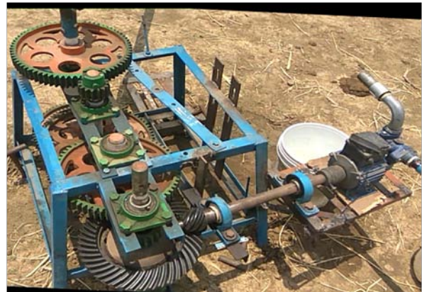
Fig. 2.4: Speed increaser with centrifugal pump.
